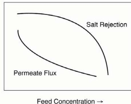
Figure 5 demonstrates that, if feed pressure remains constant, higher salt concentration results in lower membrane water flux. The increasing osmotic pressure offsets the feedwater driving pressure. Also illustrated in Figure 5 is the increase in salt passage through the membrane (decrease in rejection) as the water flux declines.
