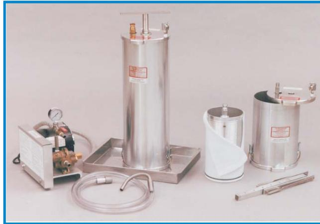
With the Lapierre syrup filter, you get a quality filtration for a maple syrup of an excellent limpidity. The filtration vessel is fast and easy to take a part when replacing the filtration cloth. The syrup filter vessel is available in 12" an 24" lenght.
